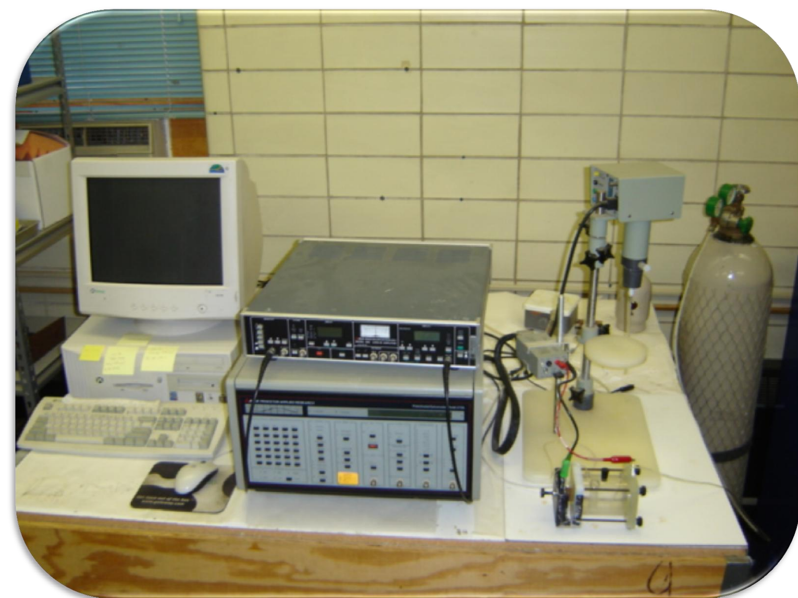
Figure 1: Image of Potentiostat and Flat Cell Apparatus
