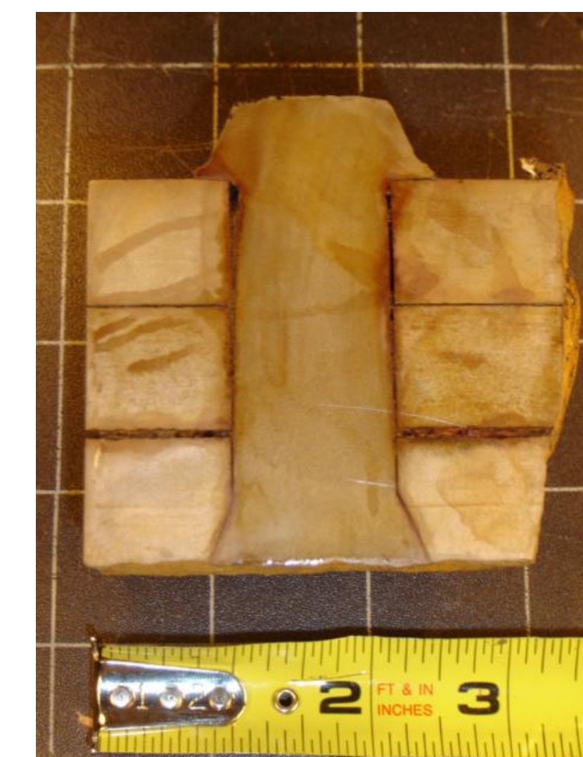
Figure 2: Macroetch of Plate A-6
